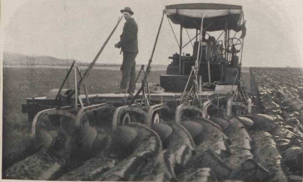
Breaking Virgin Sod. Eight, 14 Inch Furrows 8 inches deep. S. A. Wright, Dunkirk, Montana
