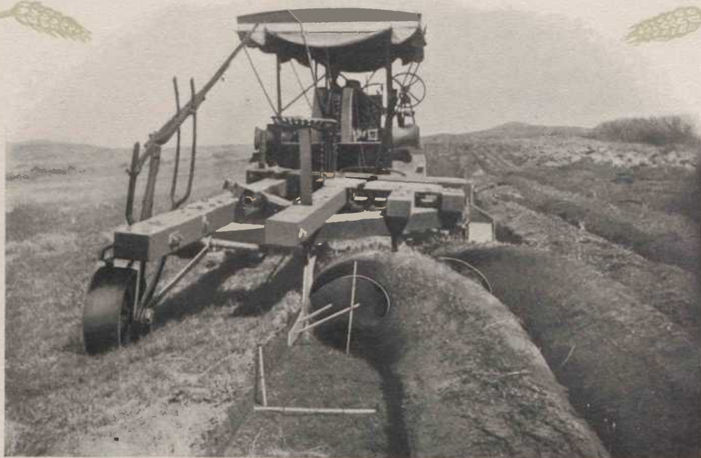
In Virgin Soil, pastured since reclaiming. Pulling 2, 24 inch Plows, at a depth of 12 inches
