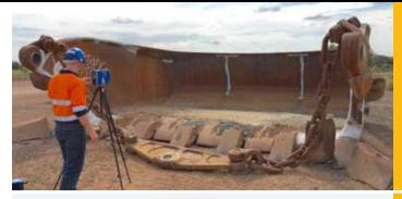
Laser scanning your bucket or blade ensures your wear package matches your equipment just as if it arrived right out of the factory.
