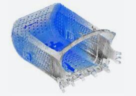
The "scan" becomes a 3D images of your bucket or blade This modeling process allows us to provide an exact fit of your wear kit on your worktool.
