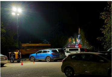
Light towers are typically run for extended periods, so the whopping 1,000-hour maintenance interval on the Perkins-powered Allmand series will lead to fewer service disruptions during ongoing projects. And not being suddenly plunged into darkness is always a good thing – right alongside decreased downtime and a healthier bottom line for the project.
