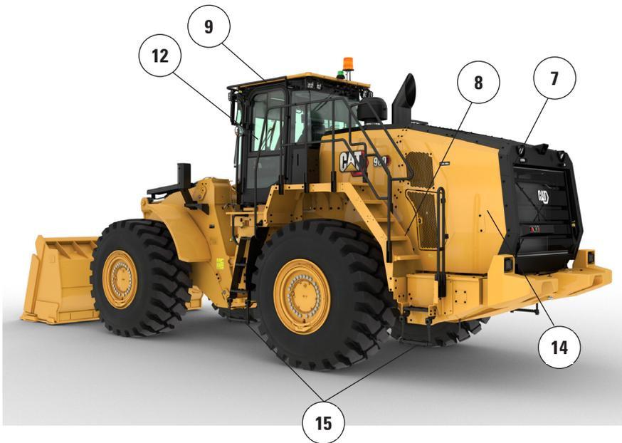
7. Ground-level parking brake override & engine shutdown switches
