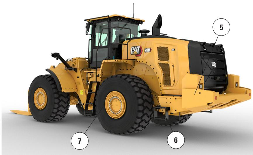
5. Heavier counterweight provides for greater tipping loads while the integrated counterweight guard protects the counterweight from impact
