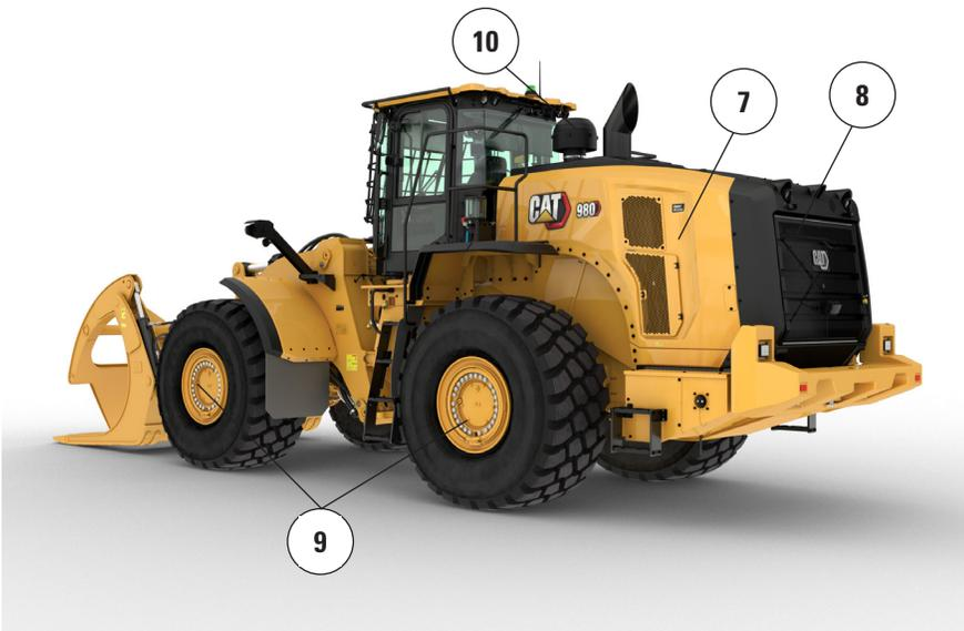
7. Optional variable pitch fan help to keep rear grill and cooling cores clean in high debris applications
