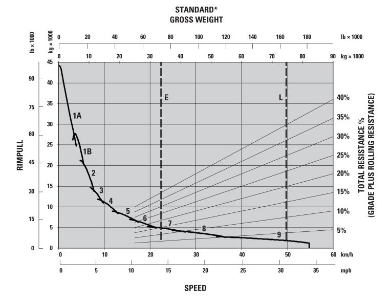
1A – 1st Gear (Converter Drive)
