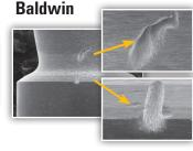
Using Cat Fuel Filters resulted in the least amount of wear on the injectors\* All the competitors had significant leak paths form as a result of erosion due to a high level of contaminates getting through the filter. As a result, engine performance and component life are greatly affected.
