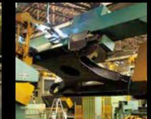
Twin welding robots make possible high-speed production of robust base frames.
