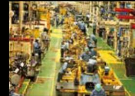
The transport interval on our 200-meter-long main assembly line can be freely adjusted based on the model being produced.
