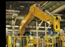
The boom/stick is quickly mounted in line with order specifications.
