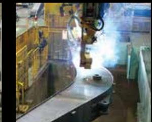
Robust frames are produced using high-speed tandem arc robot welding.
