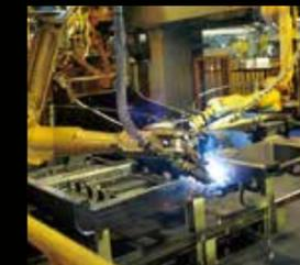
The plant's swing frame FMS consists of four state-of-the-art welding robots.
