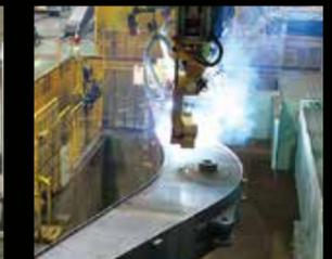
Robust frames are produced using high-speed tandem arc robot welding.
