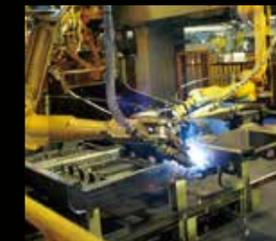
The plant's swing frame FMS consists of four state-of-the-art welding robots.
