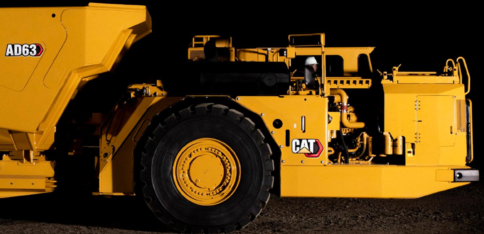
The new 63 tonne (69 tons) AD63 underground articulated truck is powered by the Cat® C27 engine that meets EU Stage V Emission Standards.
