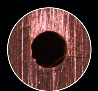
Magnified image of abrasive wear on hydraulic pump top plate.
