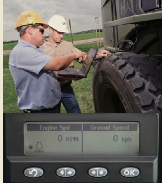
Messenger system located inside the cab.
