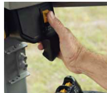
Scarifier control pod.
