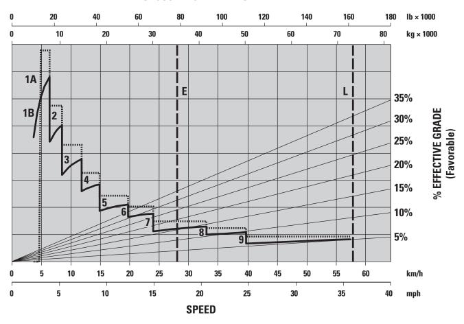
1A – 1st Gear (Converter Drive)
