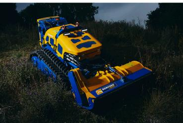
The compact, original, extra and supreme models are currently powered by Perkins three and four cylinder 400 Series engines meeting EU Stage IIIB emission standards and will soon be fitted with the latest Stage V Perkins engines built in Peterborough, UK.
