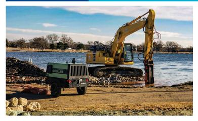
The compressor houses a 27-gallon fuel tank for up to ten continuous hours of use, and the turbo-charged engine allows it to handle high altitudes. Users are covered in virtually any temperature setting, with an extreme weather operation range of -20 to 122 degrees Fahrenheit.
