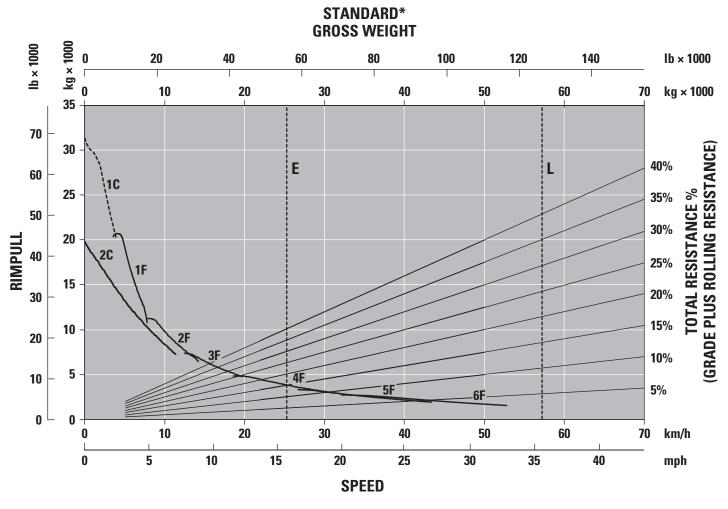
1C - 1st Gear (Converter Drive)
