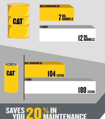
The 395's extended and synchronized service intervals, along with reduced hydraulic oil capacity, mean you'll be able to spend more time working and up to 20 percent less in maintenance costs than the previous model.
