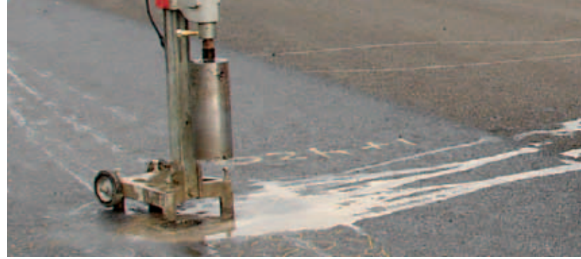
Cutting cores and lab analysis provide the final confirmation that the test strip test density meets the target.
