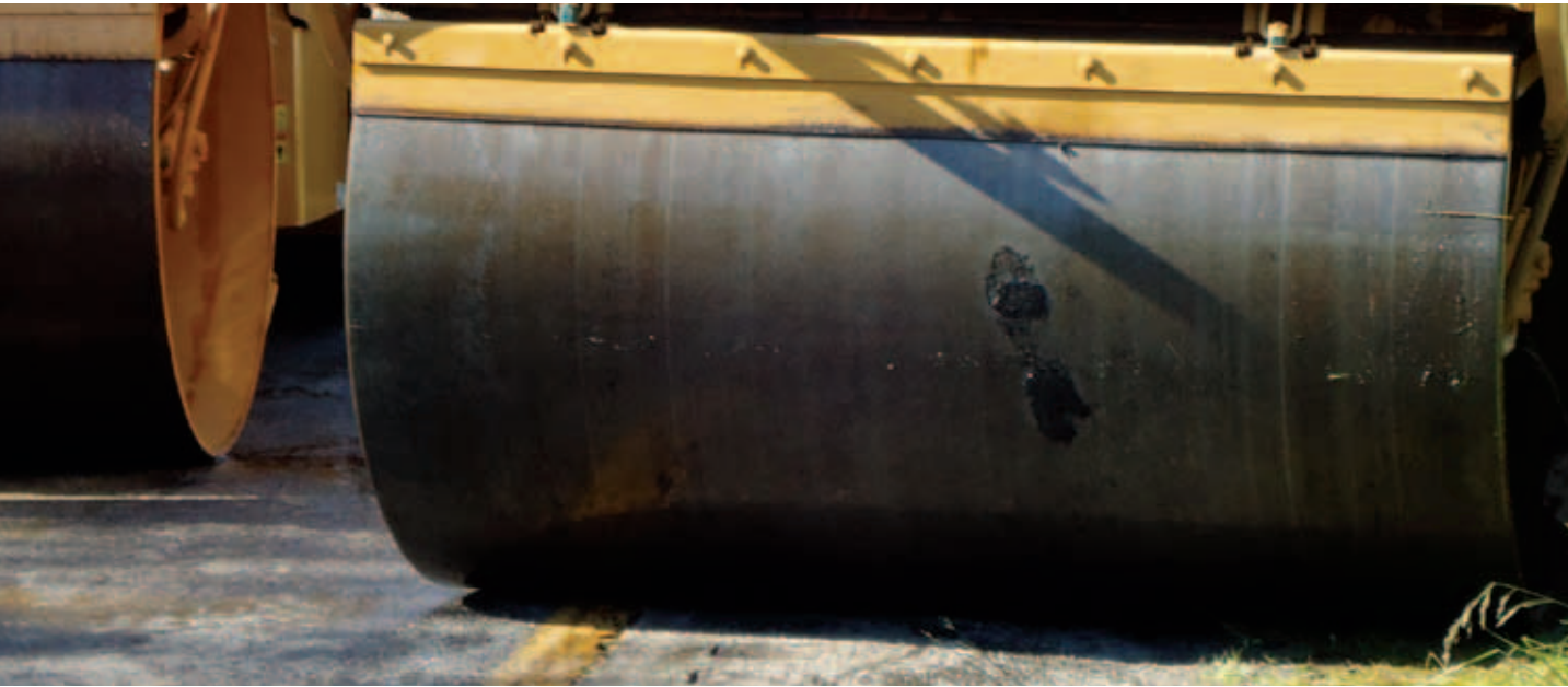
Stone Matrix Asphalt with polymer-modified asphalt cement stuck to steel drum.
