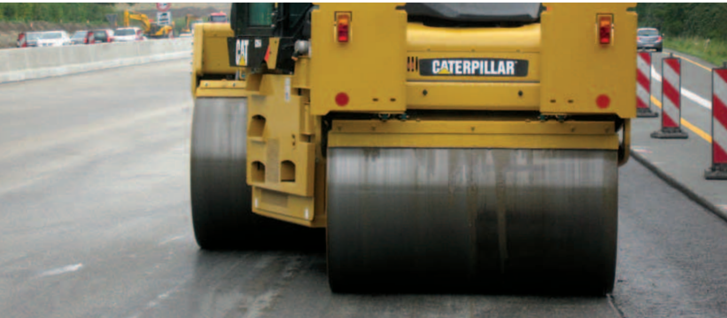
Offset drum capability facilitates wider coverage for faster compaction on thin mats that lose heat rapidly.
