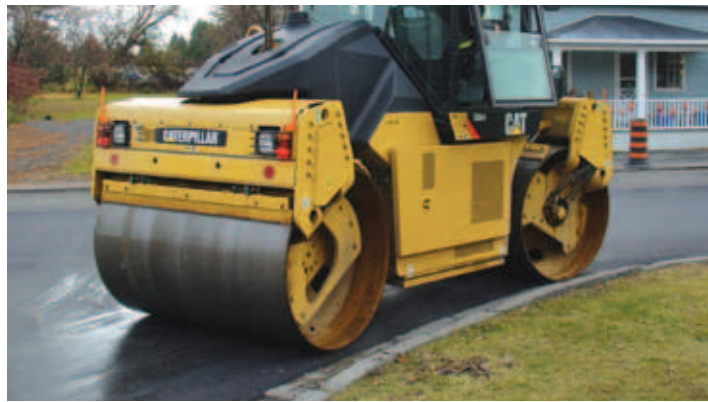
Split drum compactors can perform radius compaction without tearing fresh asphalt.
