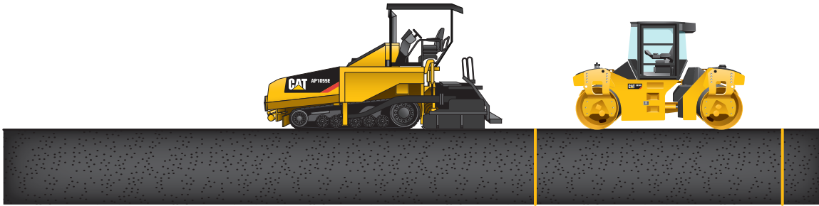
The initial phase roller works close to the paver.
