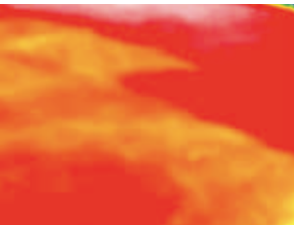
Temperature variation caused by 10-minute paver stop. Screed imprint seen in infrared image is not visible in digital image.
