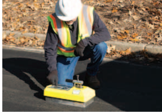
Maintaining a consistent pattern and consistent density behind the paver can be challenging.
