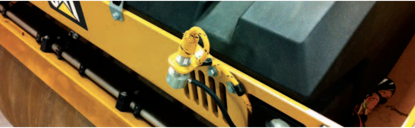
Infrared sensors send temperature data to the display in the operator's compartment.
