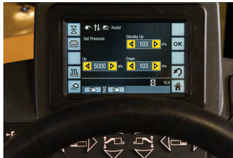
Screed counterbalance is a standard feature on Cat Pavers.
