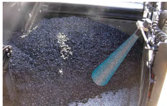
Sonic sensors should be positioned perpendicular to the moving head of material.
