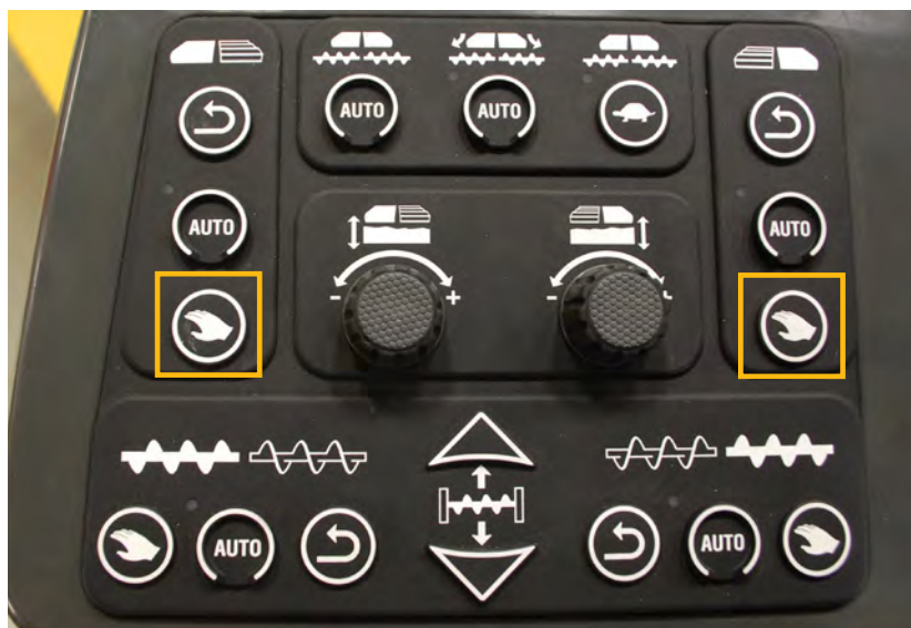
Fill the auger chamber using manual conveyor and auger controls.
