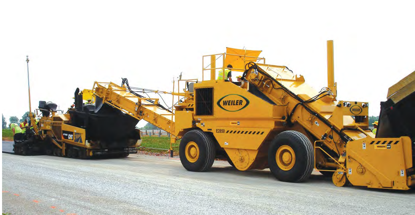
Larger material transfer vehicles have more storage capacity.
