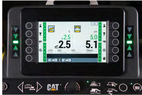
Dual screen mode showing elevation (grade) control right side and slope control left side
