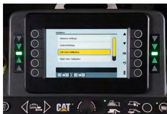
Display showing the start of calibration for the left tow-point valve.
