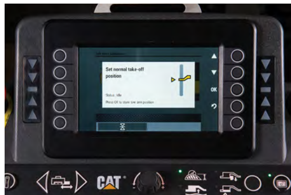
Display with instruction to set the lower limit of tow-point travel.
