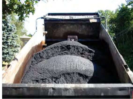
Break the load and watch for signals to raise the bed.
