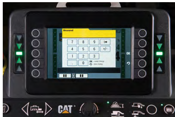
A keypad displays when the measured value is selected.
