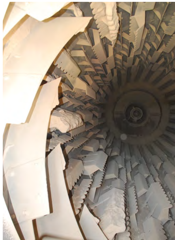
A drum mixer's spiral flights continuously moves aggregate to the lower end.
