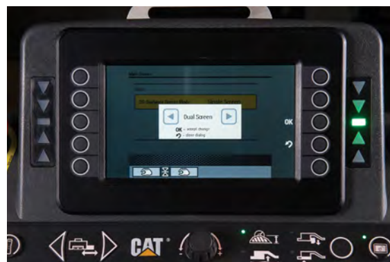
In the Operator Settings menu, an operator can set single screen or dual screen display.
