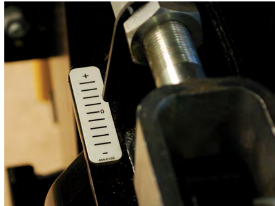
Thickness control scales are located on both sides of the screed.
