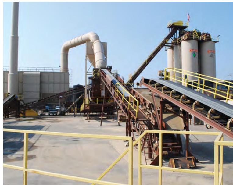
The feed system is designed to deliver a steady flow of aggregate to the mixer.
