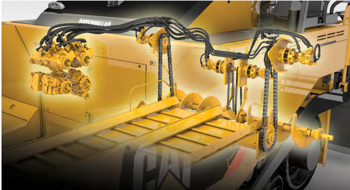
Left and right feed system conveyors move material to the front of the screed. Left and right augers move material out to the full paving width.
