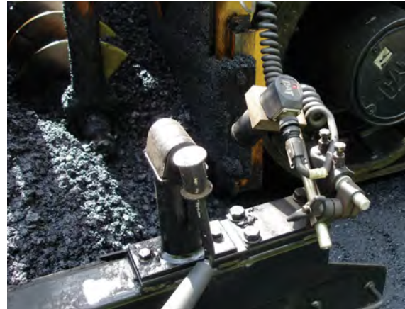
Sonic feeder sensors emit sound pulses that rebound off the material coming out the auger chamber and back to the sensor.
