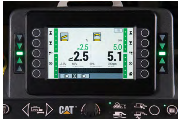
The display serves as a slope monitoring system at all times.
