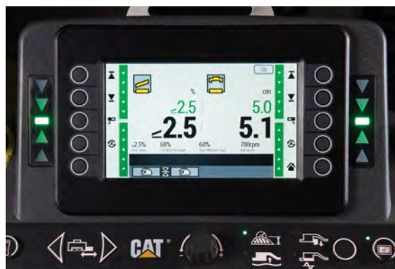
Bench the system and the target value will match the measured value.
