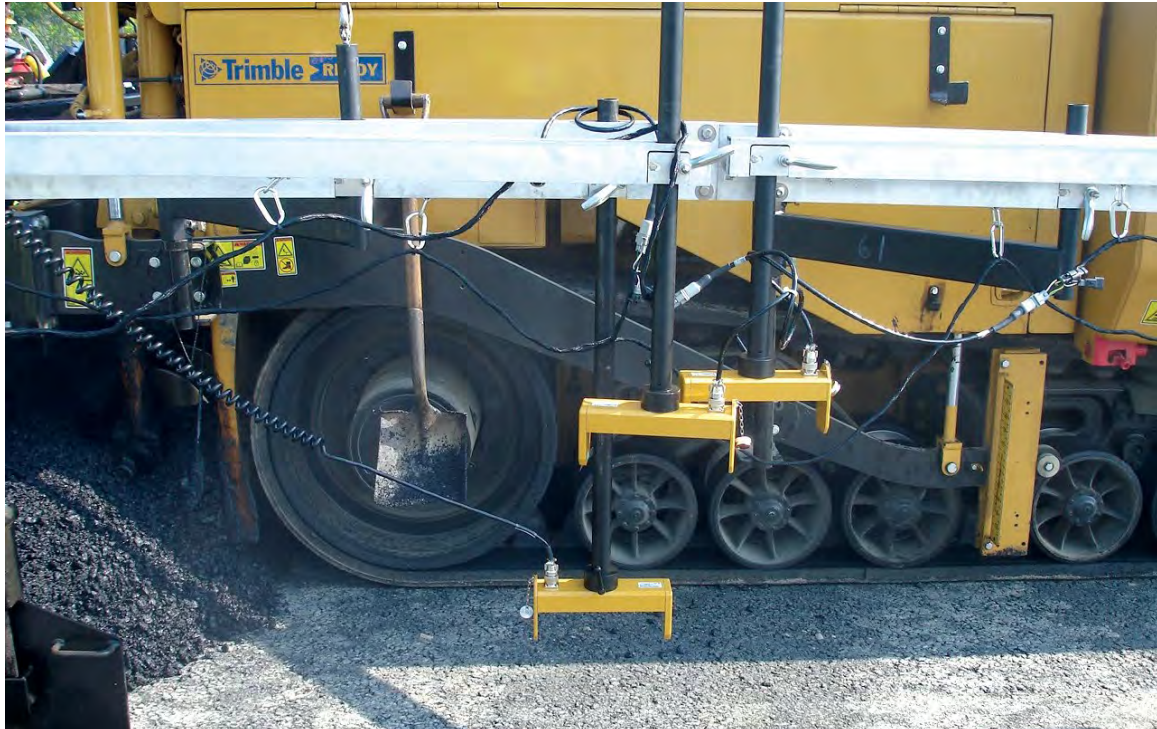
Cat non-contact averaging ski with end sections folded and set up to use only the center sensor for a single sensor application.
