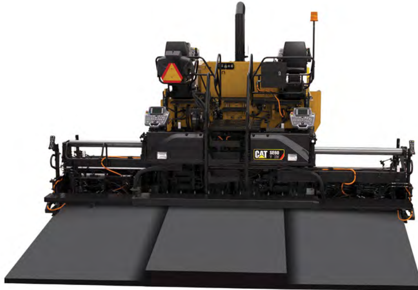
Extender height is too low
