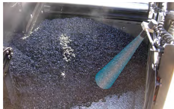
Sonic feeder sensors should be aimed at the active head of material coming out of the auger chamber.
