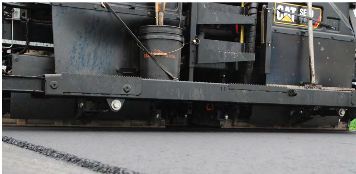
When the planing angles are the same on the main screed and the screed extenders, the texture of the surface is uniform.
