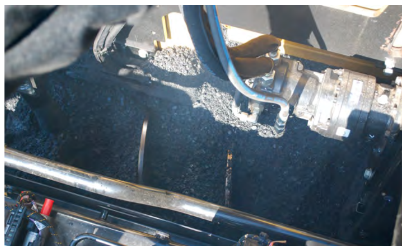
Observe the head of material in the center of the auger chamber.
