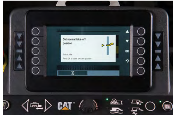
Display with instruction to center the tow-point.
