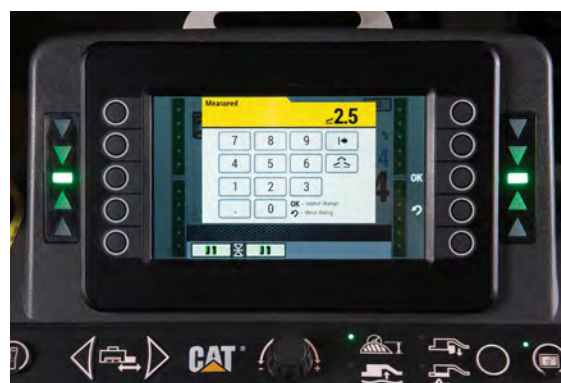
Calibrate the slope sensor with the measured slope.
