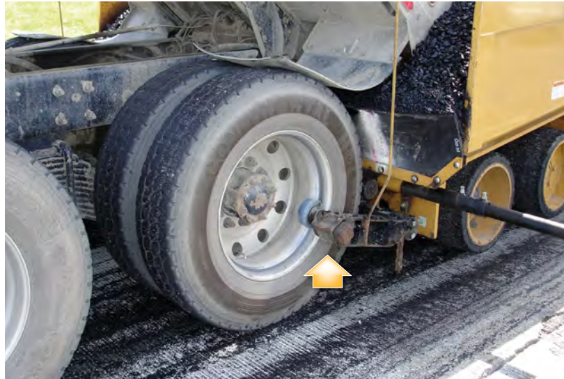
The optional truck hitch helps provide a secure connection between the front of the paver and the haul unit.
