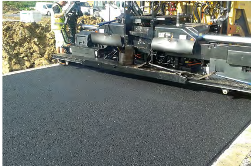
Rear-mount extendable screeds have extenders that move in and out behind the main screed.
