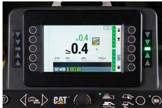
The word "AUTO" appears when the automatic mode is selected.
