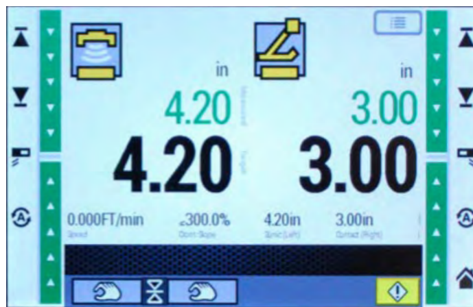
Set the Grade Control system before pulling off the starting reference.
