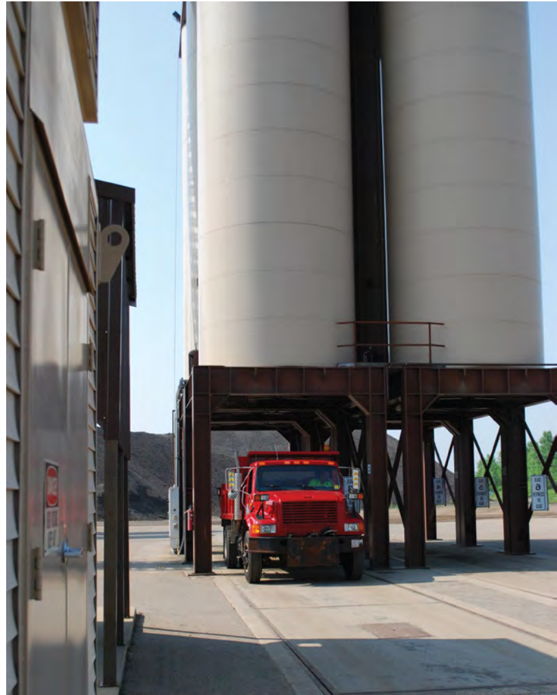
Surge and storage bins help assure uninterrupted flow of material to the worksite.
