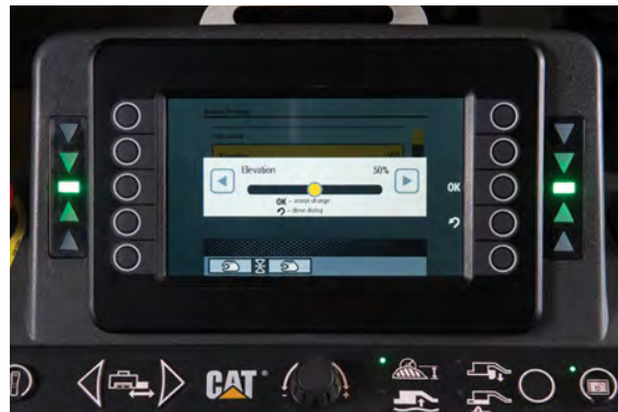
Increasing the value of the Elevation Valve Speed also speeds up screed reaction.
