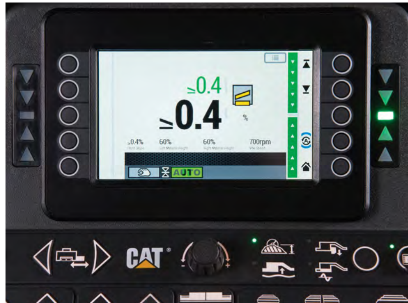
Use the display or control box to slowly make slope changes.
