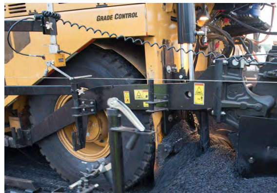
The mechanical sensor can be equipped with a wand that traces a stringline over an averaging ski.
