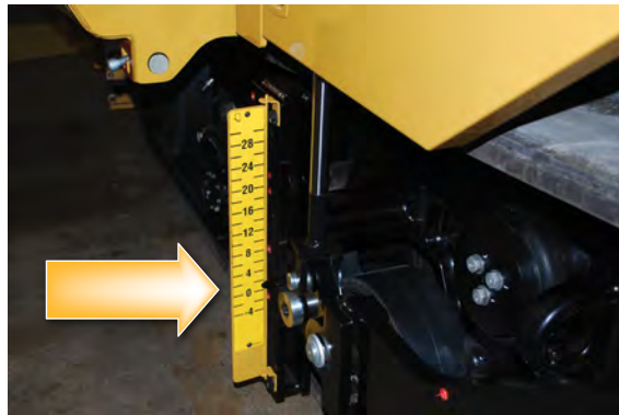
Set the tow-point height to create the correct line of pull.
