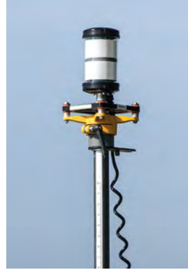
Machine targets on the paver are tracked by the Universal Total Stations.
