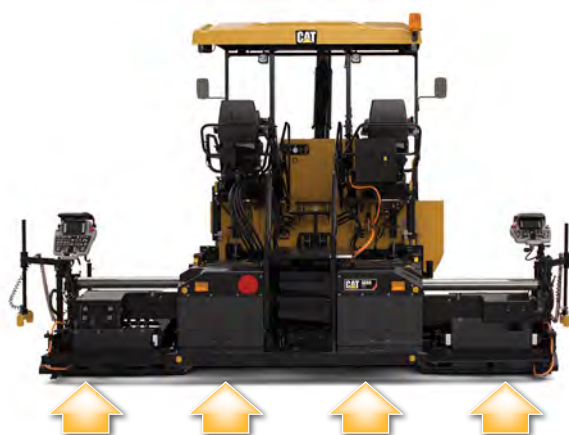
Boards should be placed at the outer edge of the main screed (behind the tractor) and outer edges of the extenders.
