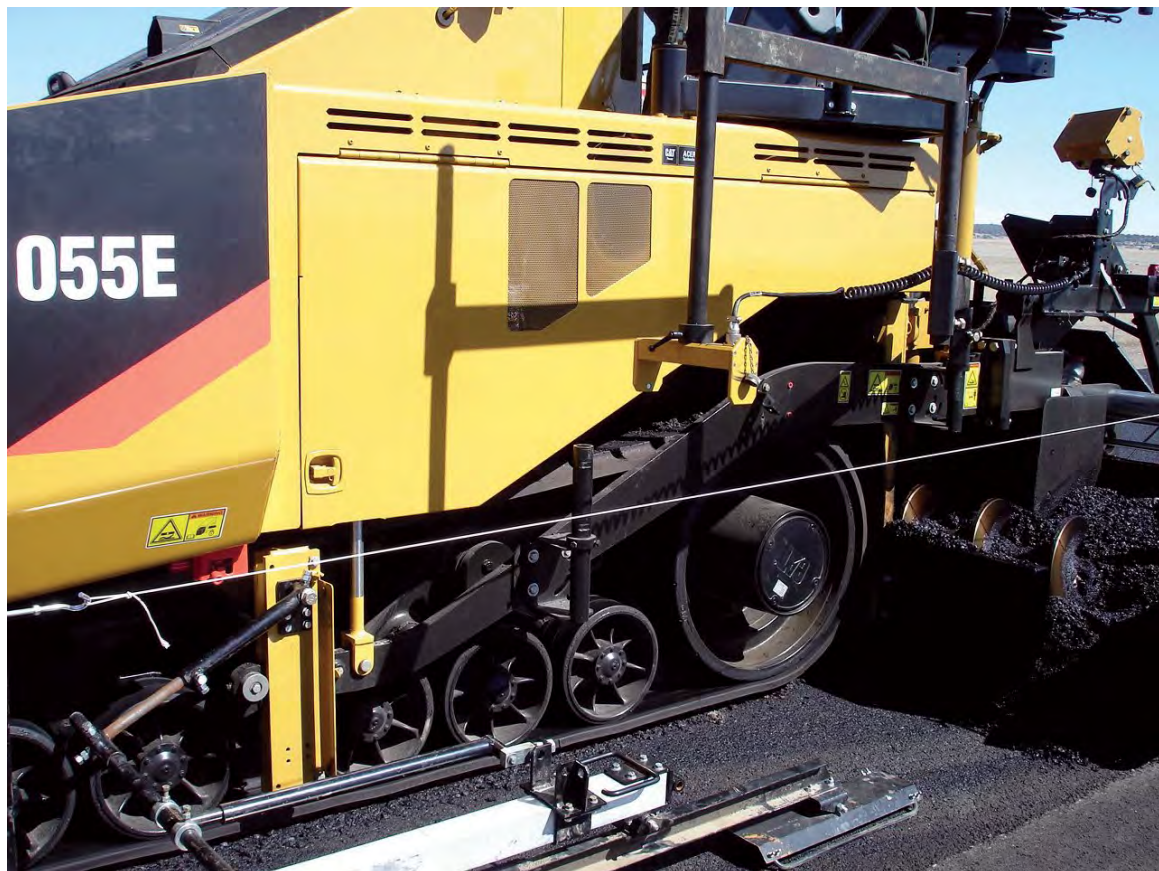
Cat sonic grade sensors are oriented horizontally when reading a stringline.
