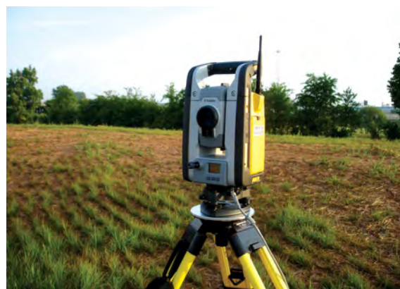
A Universal Total Station provides off-machine guidance feedback for the paver.
