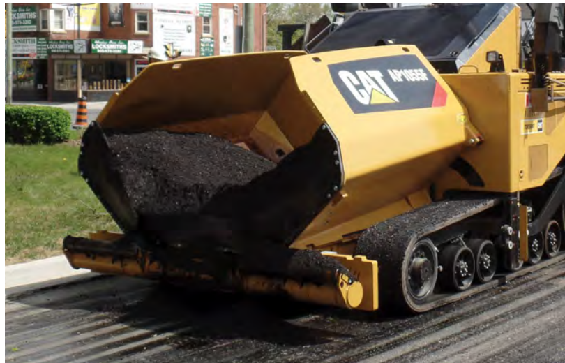
The operator can raise the sides of the hopper, if desired and permissible, to move mix from the sides of the hopper to the feed system conveyors.
