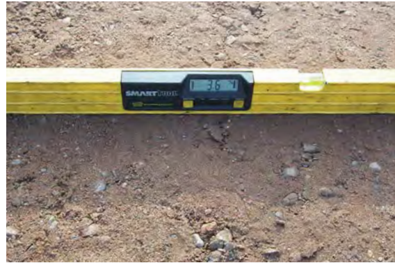
Electronic slope meter showing 3.6 percent slope from right to left adjacent to where the grade stake on page 221 shows 4 percent required.
