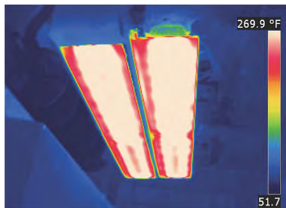
Infrared image of screed plates heating with electric screed heat
