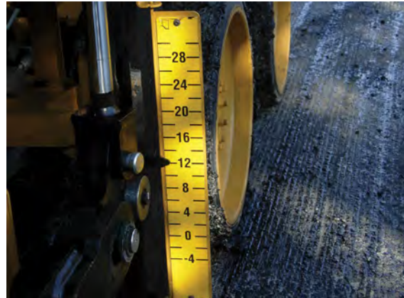
The tow-point connection features a height scale that enables the tractor or screed operators to set and check the position of the connection.
