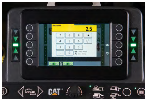
Keypad showing 2.5 inches entered as the measured value.
