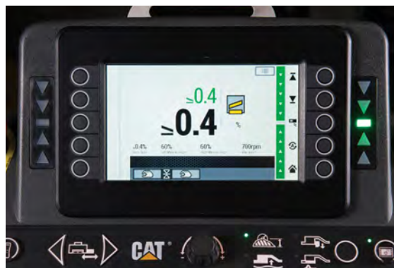
The green on-grade bar illuminates when the system is benchmarked.
