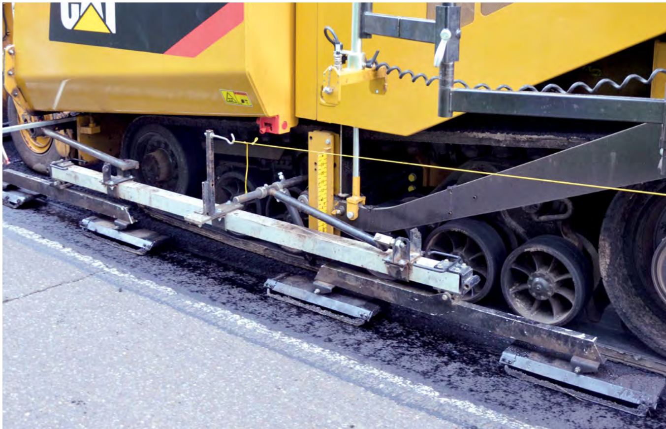
Mechanical ski is the better choice when there is a high degree of roughness in the grade to be paved.
