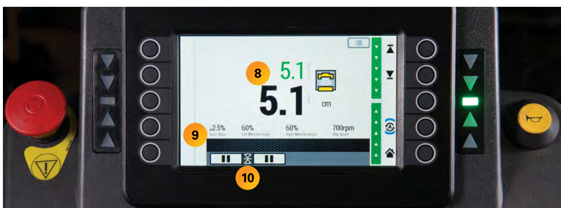
Touching the Sensor Selection icon opens the sub-menu of available sensors.
