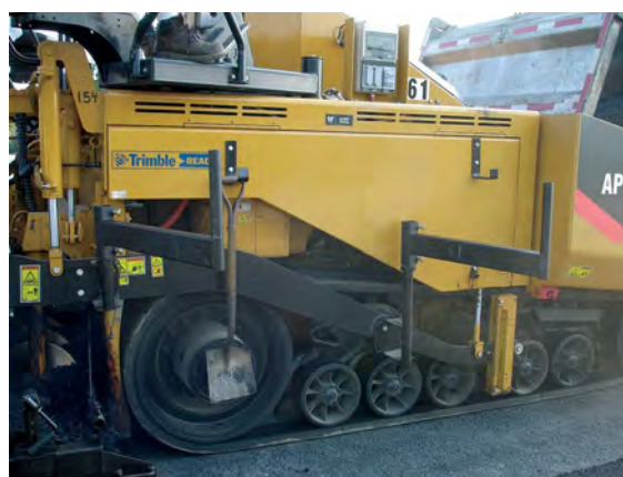
Two mounting arms, either single or scissor-type, attached to the tow arm carry the non-contact ski.
