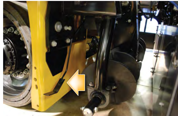
When swung out to a 45-degree angle, the tip of the paddle should be about 45 cm (18") away from the last auger segment.
