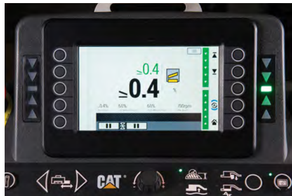
The Pause symbol will alternate with the word Auto when the propel lever is in the Neutral position.
