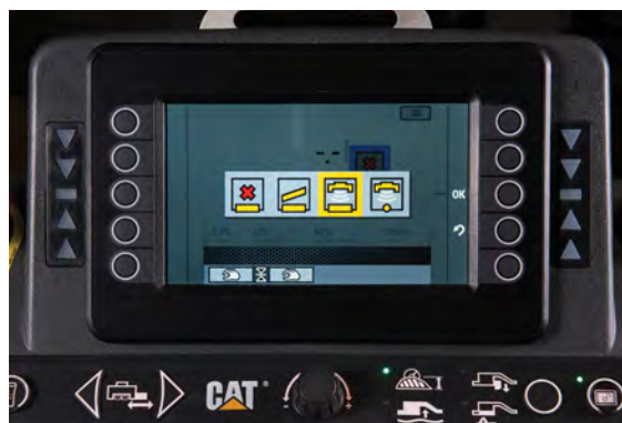
Touching the Sensor Selection icon opens the sub-menu of available sensors.
