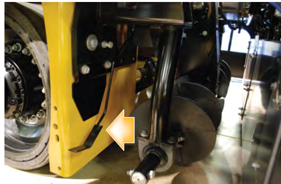
Paddle sensors provide accurate control and are easy to adjust with a measuring device.
