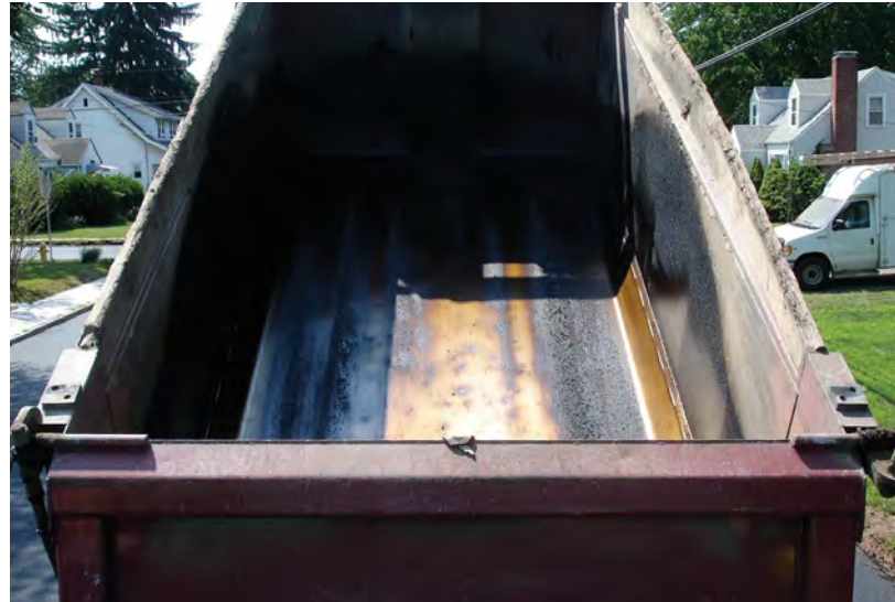
Truck beds require periodic application of approved release agent.
