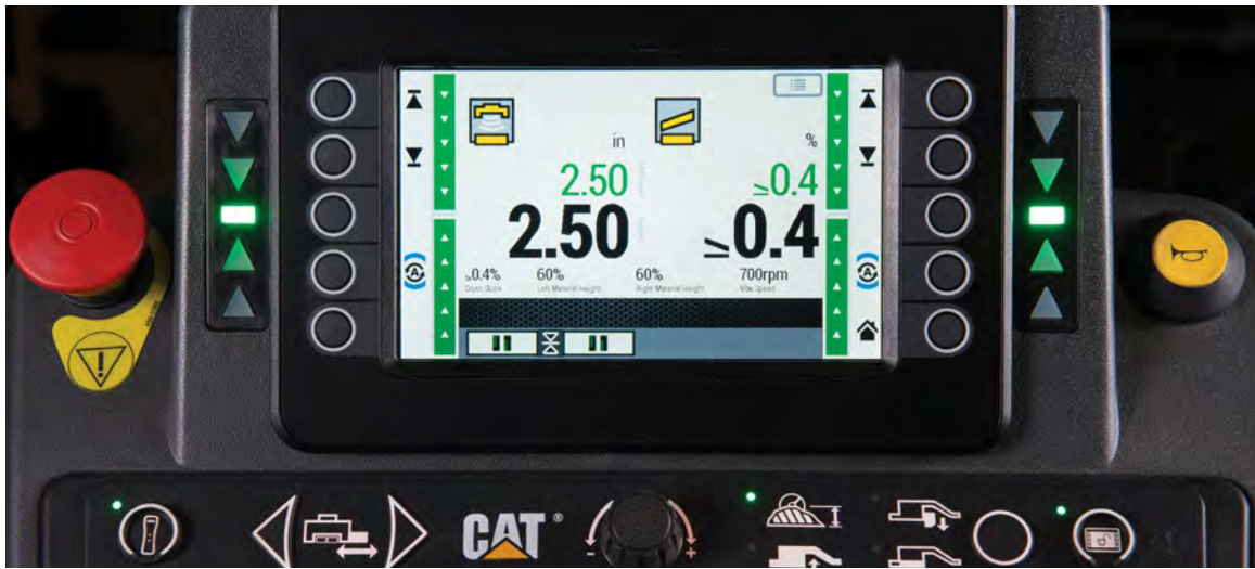
Dual screen display with single sensor grade control left and slope control right.
