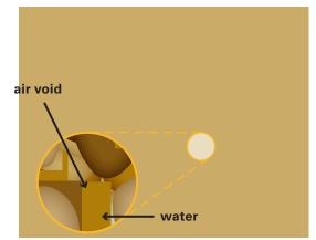
water. When a soil material has too much air and water due to abundant voids, the soil will be unstable. The process of compaction rearranges the soil particles to minimize the volume and size of air voids, making the material more dense and stable.
