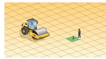
Traditional measurement systems analyze only a small proportion of the compacted area.
