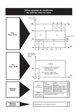
**German Soil Classification System** – DIN18196 classifies all soil materials for construction purposes into groups based on particle size according to DIN4022, mass proportions, plasticity and the presence of organic and calcareous components. Generally, coarse particles and fine particles are judged differently as coarse particles have a particlesize distribution criterion and fines have a plasticity criterion.
