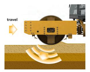
When the direction of the eccentric moment matches the direction of machine travel (top illustration), the net torque applied to the drum causes the accelerometer to sense the soil from a certain angle. When the direction of the eccentric moment does not match the direction of machine travel (bottom illustration), the torque forces change, changing the angle of measurement. This will result in consistently different CMV readings for forward and reverse operation.
