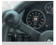
machine-integrated compaction measurement
