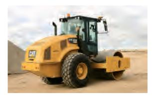
Machine-integrated compaction measurement systems provide a prediction or indication of soil stiffness.
