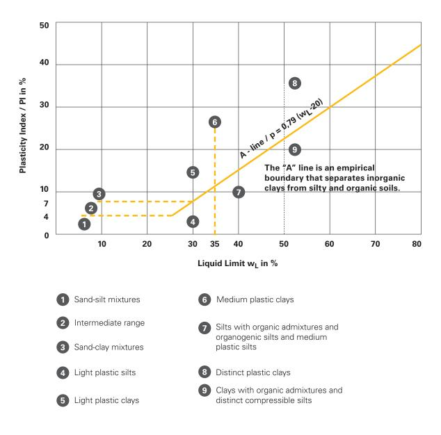
**Plasticity** refers to the degree of cohesiveness and deformable nature of a soil. The measure of plasticity is expressed as the Plasticity Index (PI). Many clay soils have a high Pl value, are quite compressible and have a high degree of cohesion. A soil with a zero PI is cohesionless or non-plastic. The moisture content of a soil also affects its PI.
