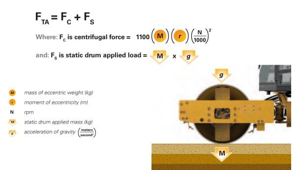
**Total Applied Force** – Total applied force is regarded as the maximum amount of vibratory energy that a compactor can apply to the ground. It is calculated by adding the static mass of the compactor to the centrifugal force. As with centrifugal force, caution should be used when using this calculation to compare the compactive capabilities of compactors.
