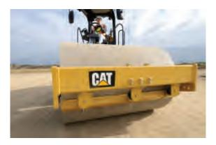
**Working Speed** – In general, travel speed plays an important part in construction productivity; the faster the machine, the faster the job is complete. However, with vibratory compactors, unlike all other types, productivity will generally increase by decreasing the travel speed. There is an optimum economical speed that will allow a compactor to achieve required compaction.
