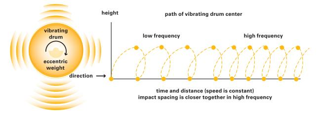
**Frequency and Speed** – Frequency is a measure of the number of complete cycles or revolutions of the eccentric weights around the axis of rotation over a given length of time. Frequency is usually expressed in units of hertz (Hz) or vibrations per minute (vpm). Typically, frequencies between 23-35 Hz (1380-2100 vpm) are used depending on material and amplitude setting.
