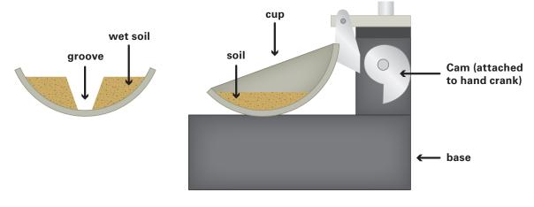
simple liquid limit testing device
