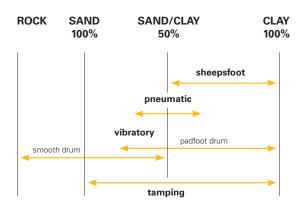
vibration. Padfoot drum machines generate the same forces, plus they also generate manipulative force. Vibratory compactors provide uniform compaction throughout the lift.
