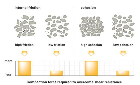
**Shear Resistance** is the resistance the soil particles have to sliding across each other when a force is applied—for example, vibration or compaction force. The shearing strength of a soil is the result of internal friction (resistance to sliding over each other) and cohesion (attraction to each other). Irregularly shaped particles have higher shear resistance than smooth shaped particles. The greater the shear resistance, the more compactive force is required to achieve density.
