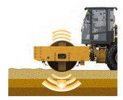
Vibratory energy is imparted on the soil by the vibrating drum.
