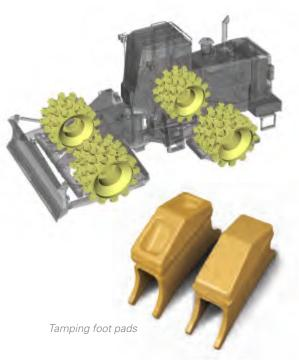
**Tamping Foot Compactors** – Tamping foot compactors are high-speed, self-propelled, nonvibratory compactors. They usually have four padded steel wheels and are equipped with a dozer blade. Their pads are tapered with a rectangular face.
