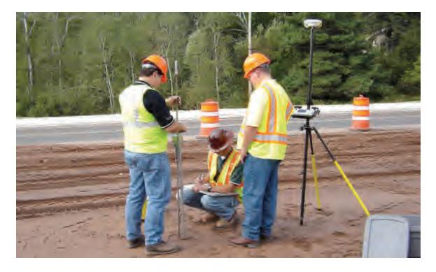
A Dynamic Cone Penetrometer in use.
