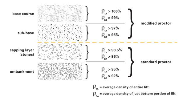
This illustration of the gradient of compaction compares the average density of the entire lift ( $\rho_{TA}$ ) with the average density of just the bottom portion of the lift ( $\rho_{a}$ ).
