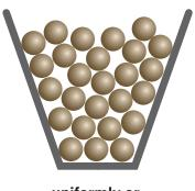
uniformly or poorly graded
