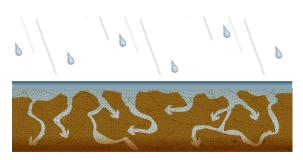
**Permeability** is the ease with which water flows through a soil. This is not the same as capillarity, which is a soil's ability to absorb water. Soil texture, gradation and the degree of compaction influence a soil's permeability. Permeability is the most variable soil parameter with values varying more than 10 orders of magnitude. Usually, coarse-grained soils are more permeable than fine-grained soils because coarse-grained soils have larger voids between their particles. **PLASTICITY**
