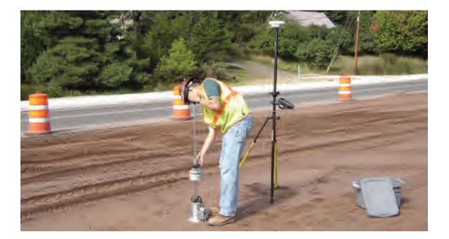
As a result, you cannot go back and get the exact same reading you obtained with a previous pass. This can pose a problem for agencies trying to verify compaction measurement values (CMV or MDP) with some other known field test for compaction.
