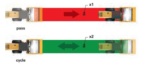
• Number of Passes – This refers to the number of times a compactor will pass over an area of ground. Caterpillar defines a pass as a single trip over an area in either forward or reverse direction and a cycle as two consecutive passes over an area, typically one in the forward direction and one in the reverse.
