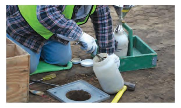
The sand cone method has proven accuracy.
