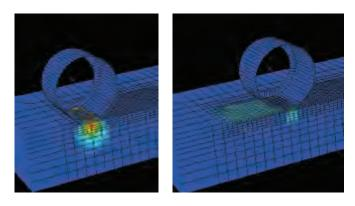
High amplitude is transmitted further into the soil.
