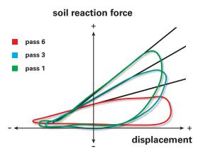
The steeper the slope of the curve, the stiffer the soil.
