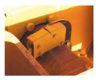
Accelerometers measure the reaction of the soil as it is struck by the vibrating drum.
