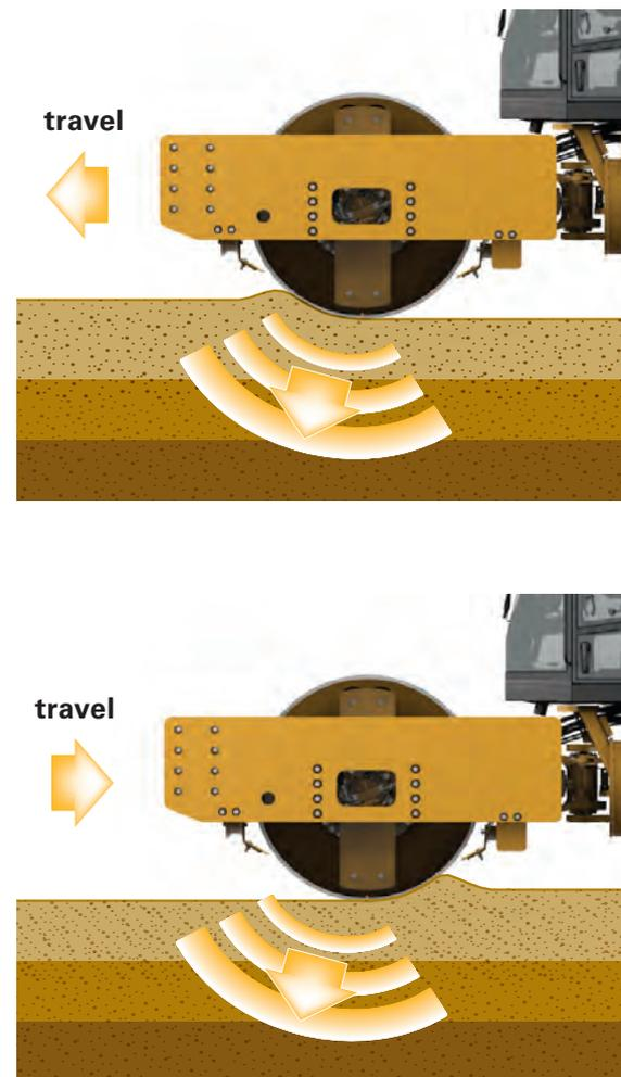
*When the direction of the eccentric moment matches the direction of machine travel (top illustration), the net torque applied to the drum causes the accelerometer to sense the soil from a certain angle. When the direction of the eccentric moment does not match the direction of machine travel (bottom illustration), the torque forces change, changing the angle of measurement. This will result in consistently different CMV readings for forward and reverse operation.*
