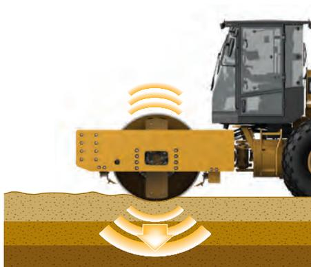
*Vibratory energy is imparted on the soil by the vibrating drum.*
