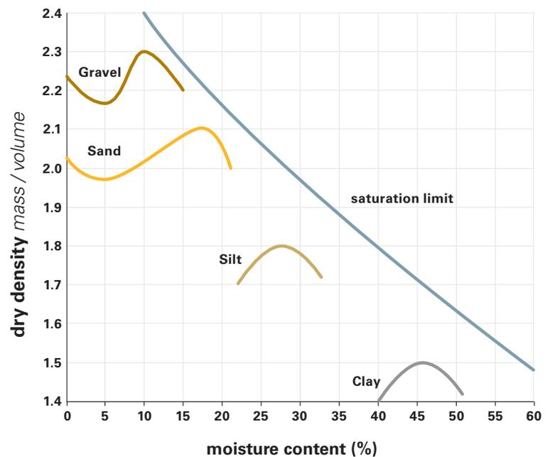
Laboratory tests determine the moisture content at which maximum density can be attained for that particular soil material. Field target densities are specified as a certain percent of the maximum laboratory dry density. Generally, required field densities will be 95 percent of Standard Proctor for embankments and up to 100 percent of Modified
