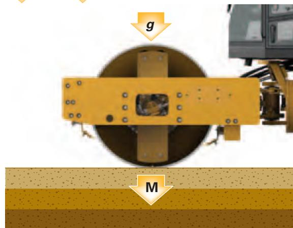
**Total Applied Force** – Total applied force is regarded as the maximum amount of vibratory energy that a compactor can apply to the ground. It is calculated by adding the static mass of the compactor to the centrifugal force. As with
