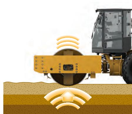
*The material vibrates in response, which is detected and measured by the accelerometer.*
