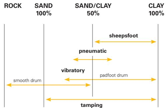
**Vibratory Compactors** – Vibratory compactors work on the principle of particle rearrangement to decrease voids and increase density and load bearing strength. They come in two types: smooth drum and padfoot drum. For increased versatility, smooth drum compactors can be equipped with optional padfoot shell kits, which allows the use of smooth drum rollers in padfoot applications, albeit with limited performance.
