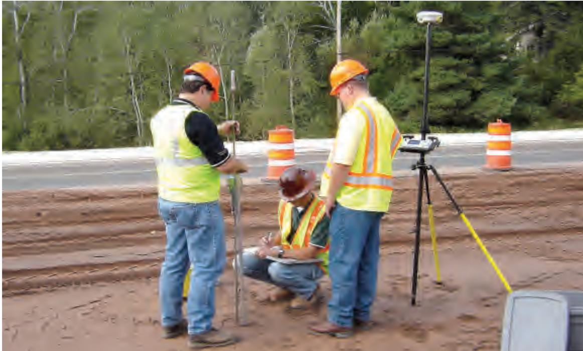
A Dynamic Cone Penetrometer in use.
