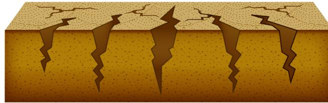
**Visible Shrinkage or Swelling** is an indication that the soil is fine-grained, such as clay. The cycle of shrinking and swelling is a result of the release and build-up of moisture within the soil. This type of soil
