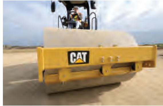
**Working Speed** – In general, travel speed plays an important part in construction productivity; the faster the machine, the faster the job is complete. However, with vibratory compactors, unlike all other types, productivity will generally increase by decreasing the travel speed. There is an optimum economical speed that will allow a compactor to achieve required compaction.
