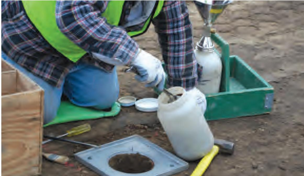
*The sand cone method has proven accuracy.*
