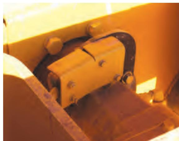
Accelerometers measure the reaction of the soil as it is struck by the vibrating drum.
