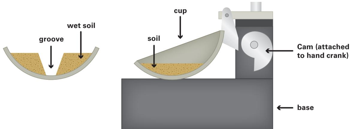
simple liquid limit testing device
