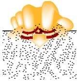
**Manipulation** – Manipulation is a compactive force that rearranges particles into a more dense mass by a kneading process. The process is especially effective at the surface of the material lift. The longitudinal and transverse kneading action are essential when compacting heavily stratified soils such as clay-type soils. Sheepfoot compactors and staggered wheel, pneumatic tire compactors are specifically designed to deliver this type of compactive force.
