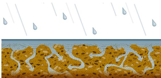
**Permeability** is the ease with which water flows through a soil. This is not the same as capillarity, which is a soil's ability to absorb water. Soil texture, gradation and the degree of compaction influence a soil's permeability. Permeability is the most variable soil parameter with values varying more than 10 orders of magnitude. Usually, coarse-grained soils
