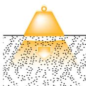
**Static Pressure** – In static compaction, pressure from the weight of the compactor produces shear stresses in the soil that cause the individual particles to slide across each other. Compaction occurs when the applied force causes individual particles to break their natural bonds to one another and reorient
