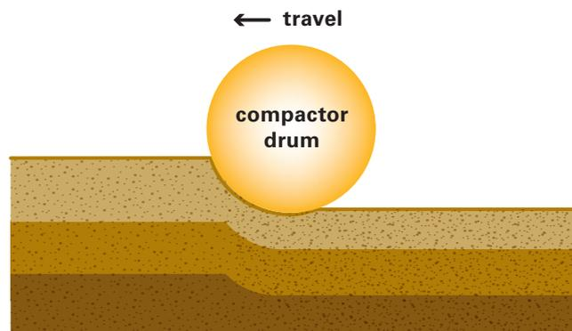
**Compressibility** is the rate of the reduction in volume of a soil when a force is applied to it. Soils with high compressibility have particles that easily reorient themselves to reduce the space available for air or water voids. In wet conditions, clay soils usually have higher compressibility than granular soils. But they have less permeability, which makes
