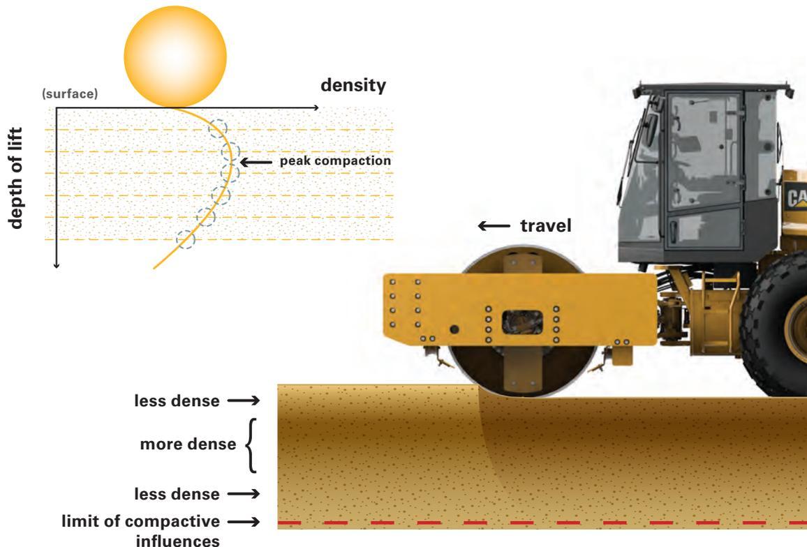
*It seems logical that when using a rolling compactor, surface soil should be the most dense— however, the peak density actually occurs below the surface, and decreases as depth lessens the influence of the compactor. This is called the Gradient of Compaction.*
