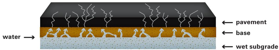
**Capillarity** is the ability of a soil to force water upward or laterally. A desirable characteristic for base material used as a layer between the subgrade and the pavement of a roadway is to act as a capillary barrier preventing upward capillary movement of water from the subgrade. Granular base also allows water to drain out of the subgrade. Capillary water is held in small pores or voids in the soil. It is considered free water, but it can only be removed by lowering the water table, heavy
