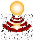
**Vibration** – Vibration is perhaps the most complex and cost-effective compactive force. More than 90 percent of the compactors sold in today’s market are vibratory. This is because vibratory compactors can produce at the same rate as a static compactor that has about three times more mass. Vibratory energy makes a vibratory compactor more efficient than a comparably sized static compactor.
