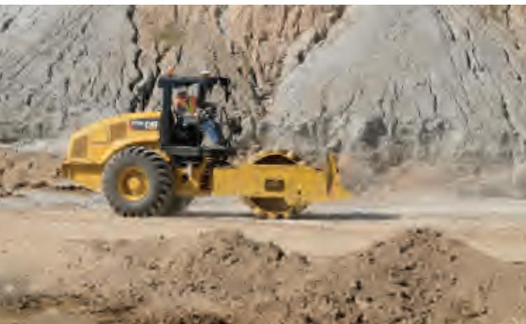
It is important to note that more recent definitions of intelligent compaction are clearly defining not only the capabilities of integrated compaction measurement and real-time display to the operator, but also the capability of recording positioning data and storing it for documentation, further analysis and records retention. As such, the definition of intelligent compaction is continually evolving.
