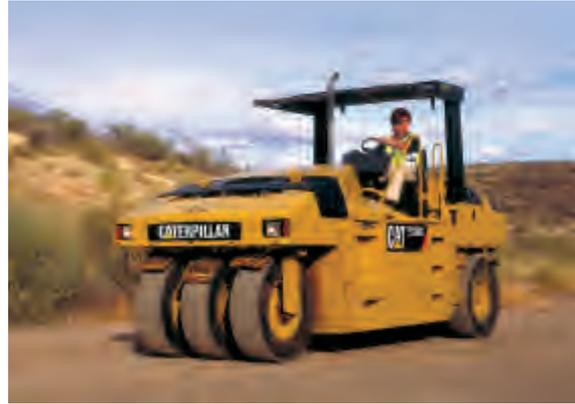
The manipulation force generated by pneumatic tire compactors is a product of two factors: the contact pressure and the wheel load. Adjusting either factor will change the performance of the compactor.
