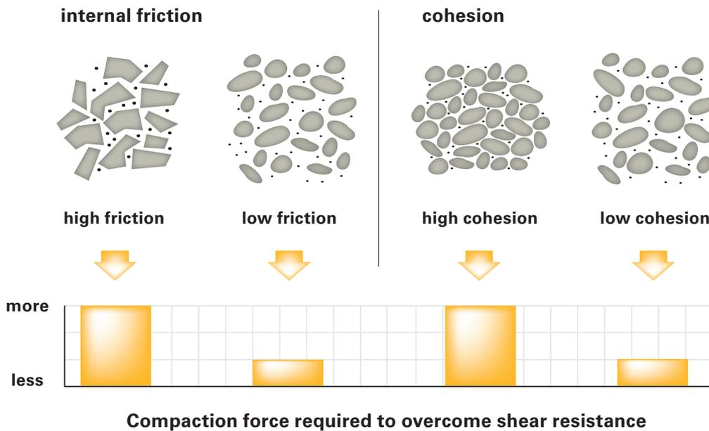
**Shear Resistance** is the resistance the soil particles have to sliding across each other when a force is applied—for example, vibration or compaction force. The shearing strength of a soil is the result of internal friction (resistance to sliding over each other) and cohesion (attraction to each
