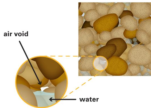
water. When a soil material has too much air and water due to abundant voids, the soil will be unstable. The process of compaction rearranges the soil particles to minimize the volume and size of air voids, making the material more dense and stable.
