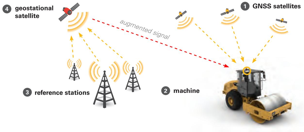
**RTK (REAL TIME KINEMATIC)**
