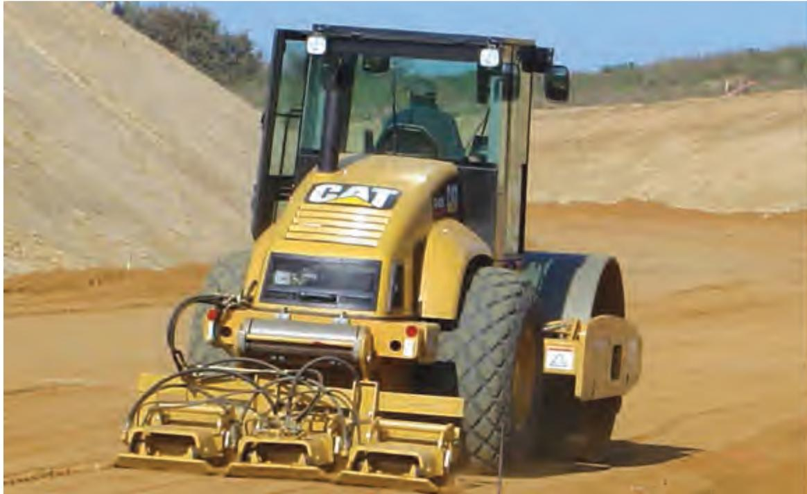
**Rear Vibratory Plates** – On non-cohesive material, single drum vibratory soil compactors can be equipped with rear vibratory plates, which provide a surface sealing that cannot be achieved with the single drum compactor alone. This enables the operator to account for the gradient of compaction: the single drum vibratory roller achieves deep compaction, and the vibratory plate compacts and seals the surface.
