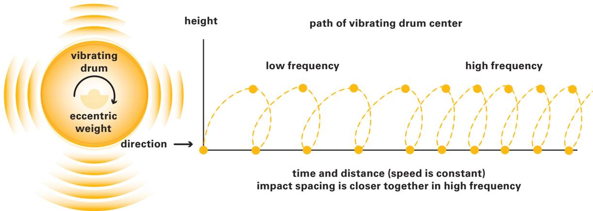
**Frequency and Speed** – Frequency is a measure of the number of complete cycles or revolutions of the eccentric weights around the axis of rotation over a given length of time. Frequency is usually expressed in units of hertz (Hz) or vibrations per minute (vpm). Typically, frequencies between 23-35 Hz (1380-2100 vpm) are used depending on material and amplitude setting.
