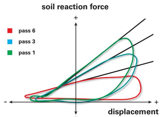
The steeper the slope of the curve, the stiffer the soil.
