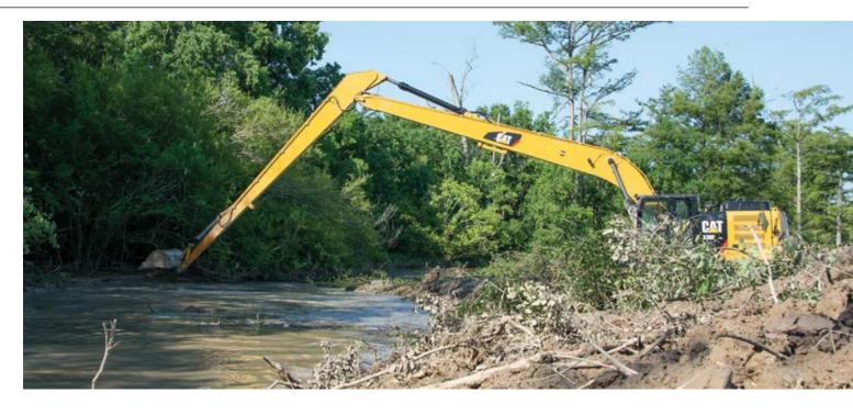
excavator, to clean out creeks, dams, parts of the Boeuf River, and ditches along roads," Evans says. "We use it to clean out Gunby Dam. It's the only machine that can reach all the way across from the levy. Trees, logs, all kinds of things get stuck in there.
