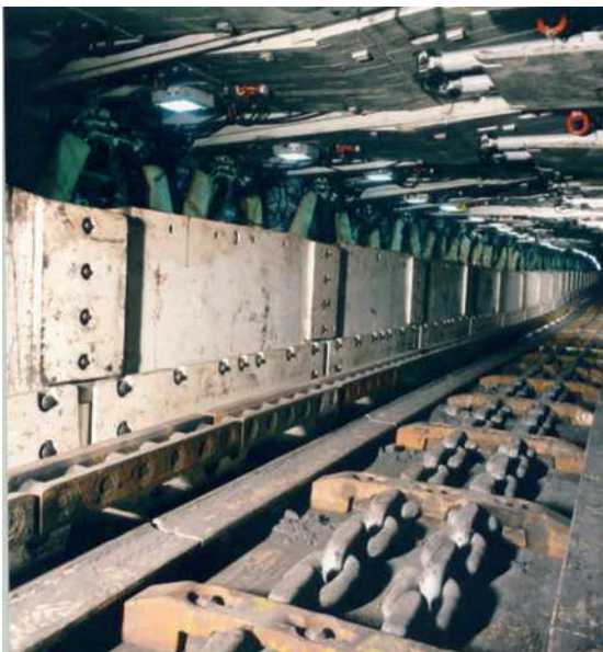
Picture 1: World's First Cat 430 m AFC Underground in Germany 1998
