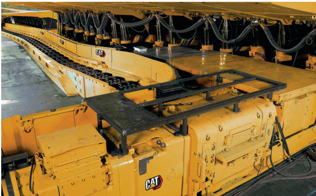
Picture 12: Compatibility Test for a Complete 400 m Long Cat Longwall
