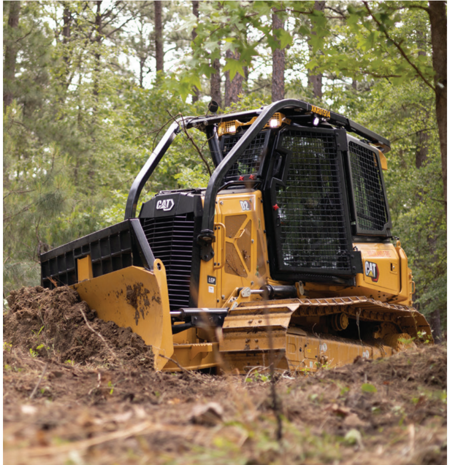
Fire Suppression Dozer
