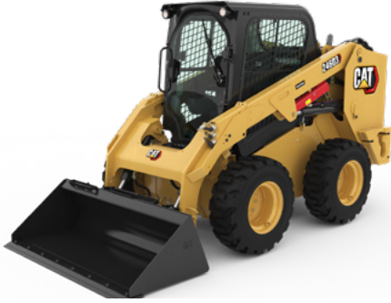
Radial Lift Linkage
