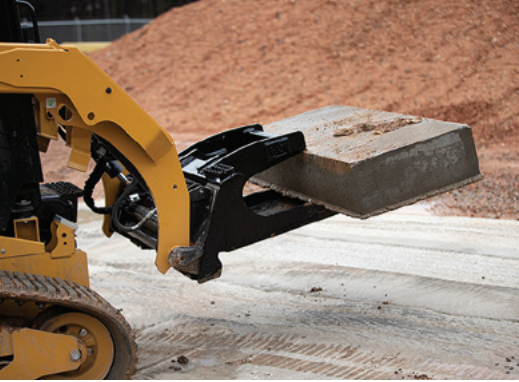
Concrete Slab Bucket
