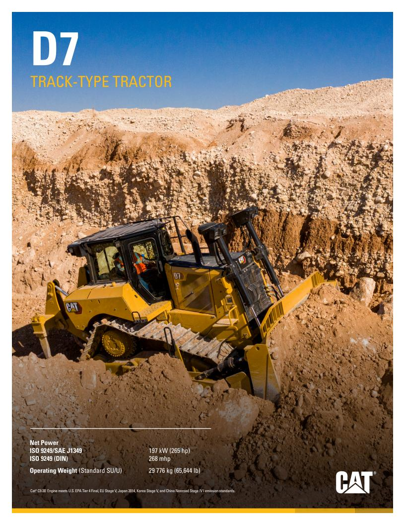
The Cat D7 joins the growing family of Next Generation Dozers, delivering more productivity and high drive undercarriage value. A fully automatic 4-speed transmission makes efficient operation easy. The broadest range of technology features in the industry work together seamlessly to help you make the most of your equipment investment.
