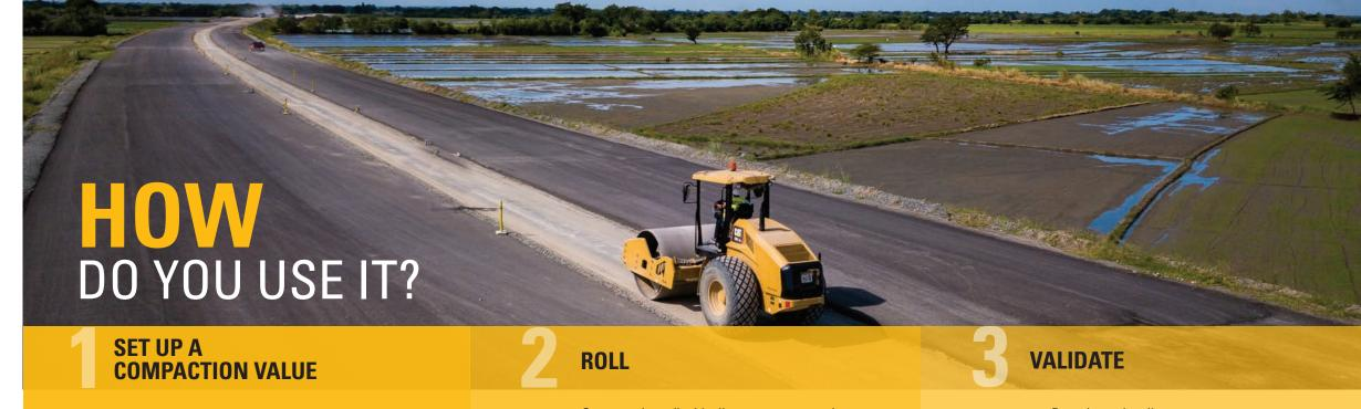
Roll a lift in a test section until the value changes less than three units each additional pass.
