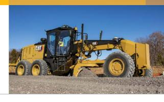
Cat® GRADE with 3D for motor graders is a machine integrated grade control system that helps you get to grade faster with more accuracy, efficiency, and productivity. Automatic blade control reduces operator inputs and the number of passes to get the job done to save you time and money.
