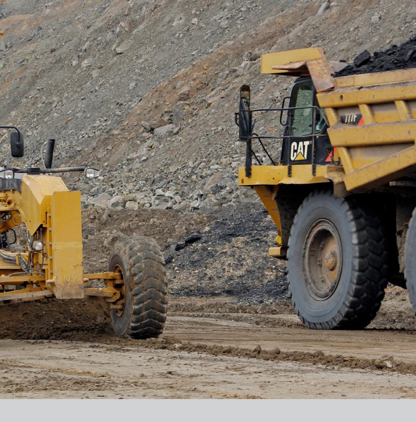
With additional power, wider moldboard and the possibility to use a more aggressive blade angle; the 18 enhances operational efficiencies by increasing coverage and reducing the number of passes required to grade your haul roads.
