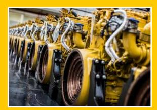
At Peterborough, we're producing the engines to meet today's challenges, and preparing for tomorrow's - all with our customers' in mind. Our manufacturing facility in Peterborough, UK produces  $Cat^{\mbox{\tiny $^{\odot}$}}$  industrial diesel engines for the compact C1.1-C.2.2, the powerful C2.8 and C3.6, the popular C4.4 and the fuel-efficient C7.1 engines.
