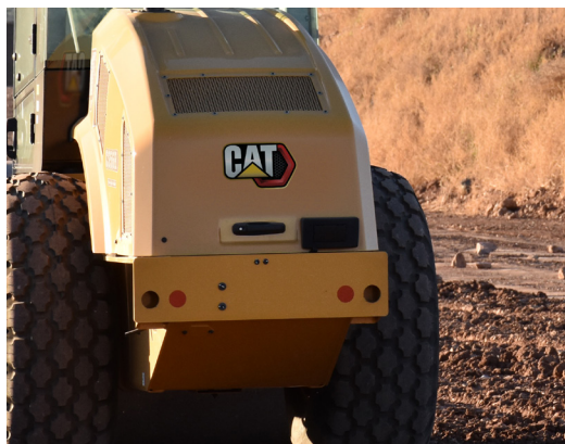
RADAR SENSOR MOUNTED TO THE REAR ENGINE ENCLOSURE.
