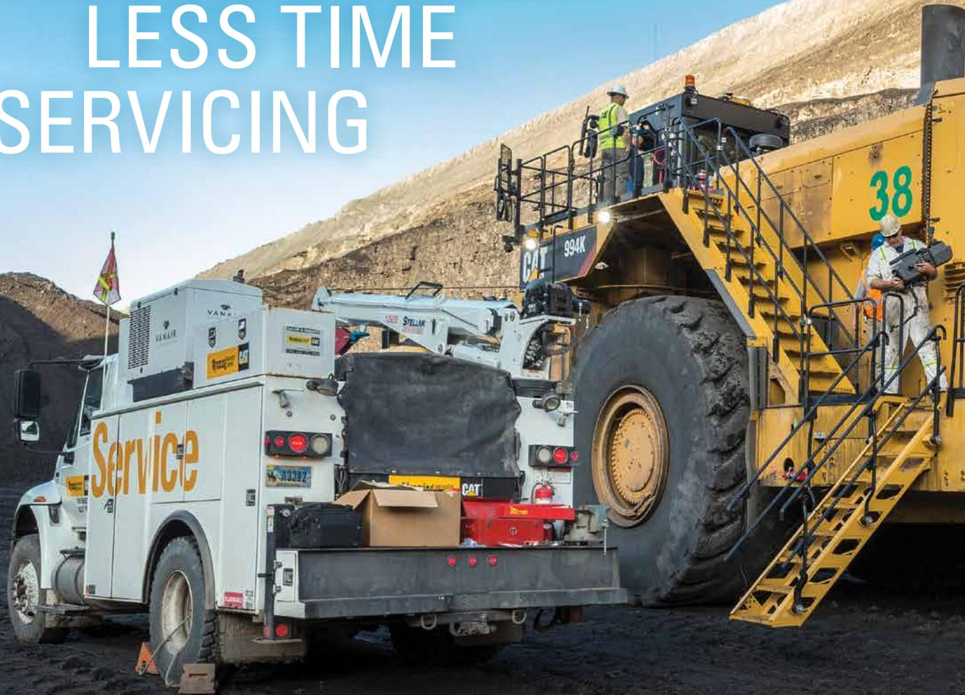
The 994K was designed to reduce the time you spend on regular maintenance procedures, with features like 500-hour engine oil change intervals and improved air filter life. The standard VIMS™ monitoring system delivers critical health and payload information, keeping performance at optimum levels and allowing advanced troubleshooting and planning to lower maintenance costs.
