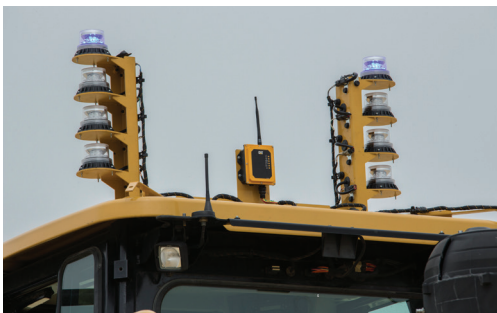
360° Visible Beacons and Roof-mounted Antennas
