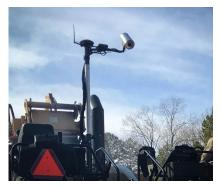
**Thermal Camera and MS955 Antenna**
