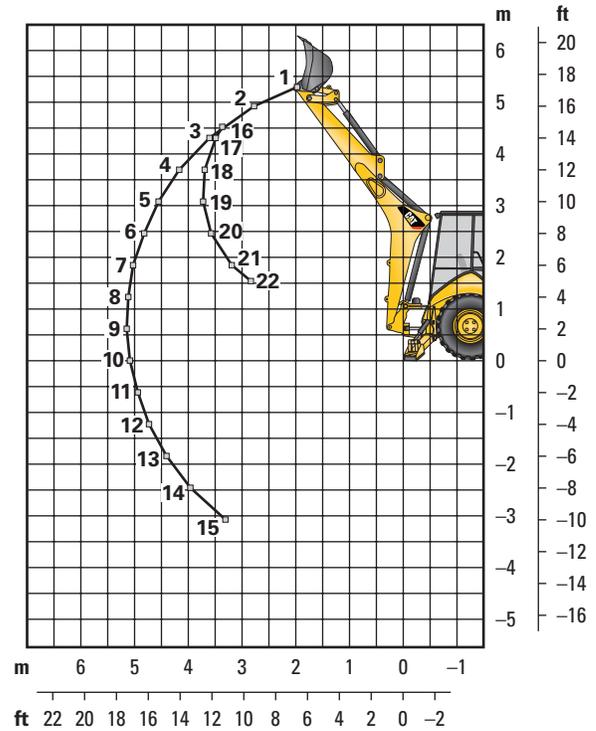
Lift capacities are over-end values calculated according to SAE J31. Values are 87% of the maximum lift force available. Machine equipped with AWD, OROPS, 0.96 m<sup>3</sup> (1.25 yd<sup>3</sup>) general purpose bucket and 460 kg (1,015 lb) counterweight. Extendible stick includes 460 kg (1,015 lb) counterweight.
