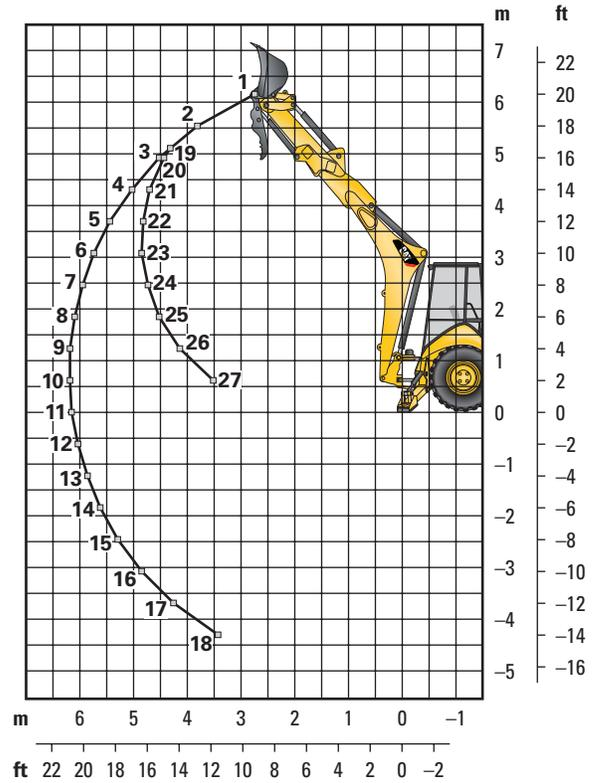
Lift capacities are over-end values calculated according to SAE J31. Values are 87% of the maximum lift force available. Machine equipped with AWD, DROPS, 0.96 m<sup>3</sup> (1.25 yd<sup>3</sup>) general purpose bucket and 460 kg (1,015 lb) counterweight. Extendible stick includes 460 kg (1,015 lb) counterweight.
