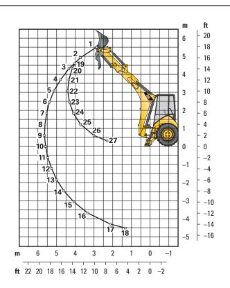
Lift capacities are over-end values calculated according to SAE J31. Values are 87% of the maximum lift force available. Machine equipped with AWD, OROPS, 0.96 m<sup>3</sup> (1.25 yd<sup>3</sup>) general purpose bucket and 240 kg (530 lb) counterweight. Extendible stick includes 460 kg (1,015 lb) counterweight.
