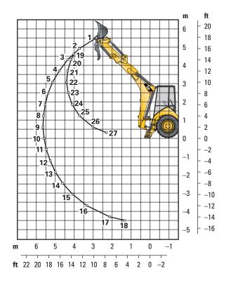
Lift capacities are over-end values calculated according to SAE J31. Values are 87% of the maximum lift force available. Machine equipped with AWD, OROPS, 0.96 m³ (1.25 yd³) general purpose bucket and no counterweight. Extendible stick includes 460 kg (1,015 lb) counterweight.
