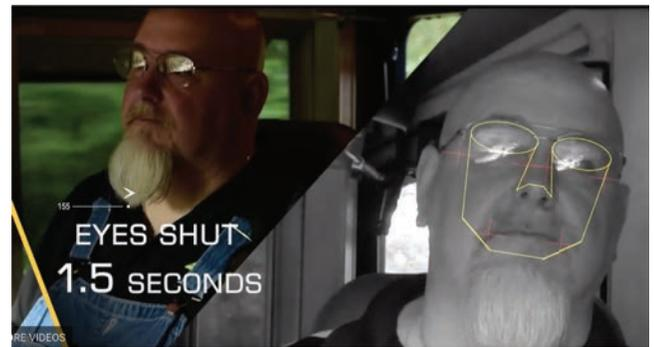
The underlying Driver Safety System (DSS) technology is based on patented eye-tracking and analytics that detects driver distraction and fatigue while on the job.
