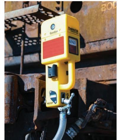
End-Of-Train (EOT) devices transmit real-time, vital information from the end of the train to the locomotive cab.
