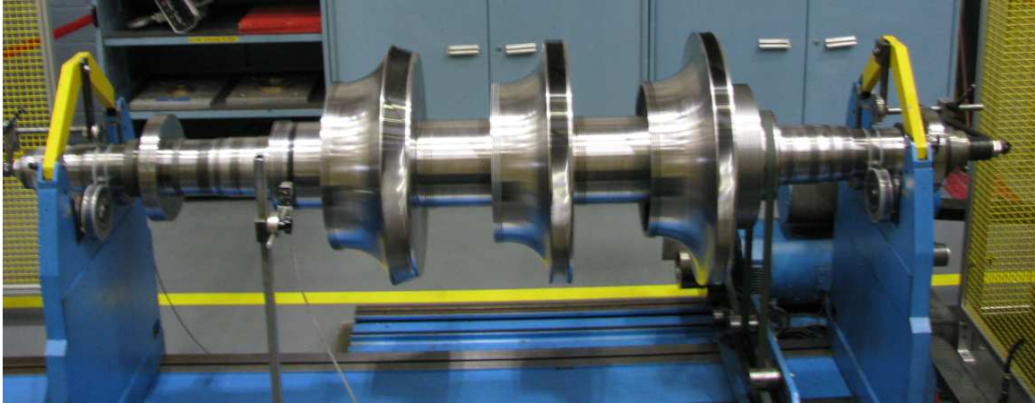
Figure 4 A typical Modular Rotor on the Balance Machine
