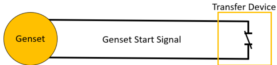
Figure 1: Generator Set Start Signal with Normally Closed Contact from Transfer Device
