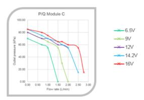
Tested over a range of voltages, high pressures on the three non-genuine pumps were still seen at low voltages. The sharp drops in pressure are symbolic of struggling pumps and increased internal slip.
