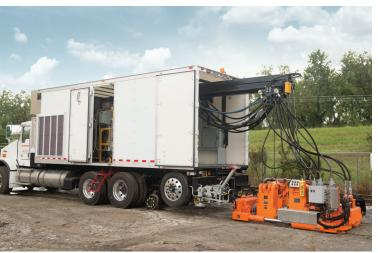
Progress Rail's Welding Division is a market leader in welding programs and equipment to improve weld performance and quality. Working with our international affiliate EO Paton, Progress Rail has developed a narrow head welder for our mobile units. This head can be used with our extended boom trucks when welding turnouts and in tight confines.
