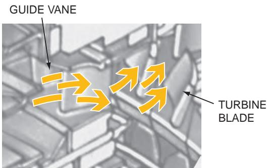
**Figure 2-14.** Gas Flow of Inlet Guide Vanes and Turbine Blade
