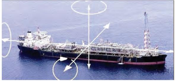
**Figure 5-5. Degrees-of-Freedom for Dynamic Movement and Static Displacement**
