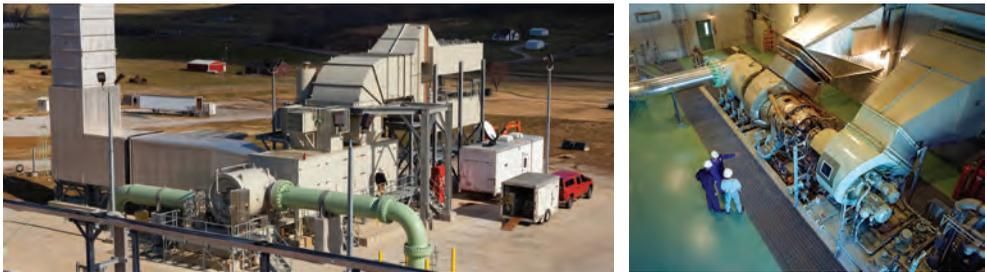
**Figure 5-1.** Gas turbine package driving a centrifugal compressor. Left: Fully enclosed, Right: Installed in a building
