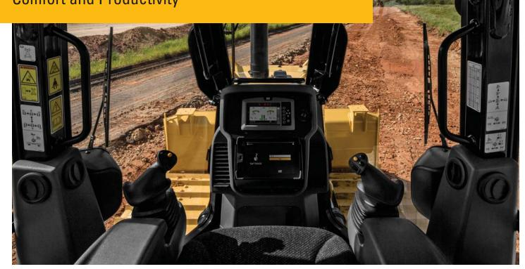
Spacious, quiet cab offers all-day comfort with wide door openings and an air suspension seat. Ergonomic, seat-mounted joystick controls isolate vibration. Excellent visibility to the blade, curbs and tight spaces help you work more precisely.
