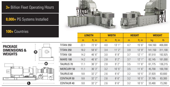
Dry weight, unenclosed height and weight. Actual values will vary depending on customer options, such as generator type. All specifications are for reference only.
