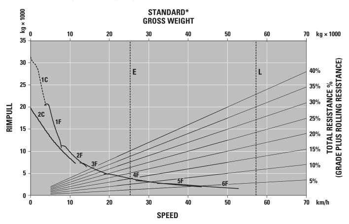
1C – 1st Gear (Converter Drive)
