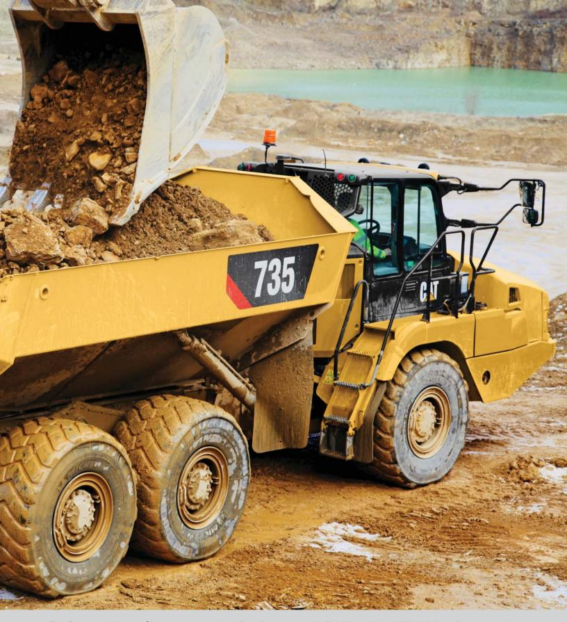
The Cat 735 with a 20  $\mathrm{m}^3/32$  tonnes capacity, offers demonstrated reliability and durability, high performance and productivity and a new world-class cab to improve operator comfort and ease of operation.
