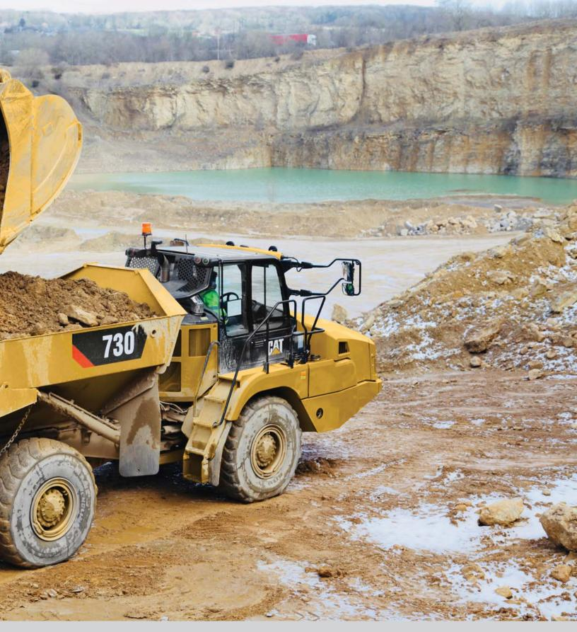
The Cat 730 with a 17.5 m<sup>3</sup>/28 tonnes capacity, offers demonstrated reliability and durability, high performance and productivity and a new world-class cab to improve operator comfort and ease of operation.
