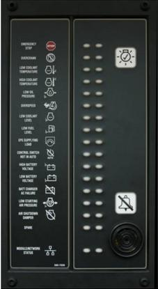
The EMCP 4 CAN Annunciator serves to display generator set system alarm conditions and status indications. The annunciator has been designed for use on the accessory communication network and may be used in either local (package mounted) or remote (up to 800 feet) application. A maximum of four annunciators may be used with a single EMCP 4.3
