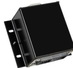
The Digital Input/Output (DI/O) module serves to provide expandable Input and Output event capability of the EMCP 4 and is capable of reading 12 digital inputs and setting 8 relay outputs. The DI/O module has been designed for use on the Accessory. Communication Network and may be used in either local (package mounted) or remote (up to 800 feet) application.
