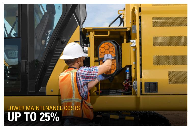
With synchronized and extended maintenance intervals, you get more done at a lower cost compared to the 330D2. Consolidated filter locations make service faster. Hydraulic, air, and fuel tank filters have increased capacity and longer life. Access to the operation and maintenance manual is easy through the in-cab monitor.
