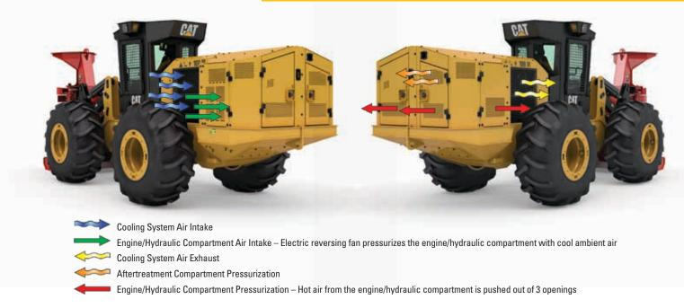
Special attention was focused on keeping the D Series cool and free of debris. The machine is segmented into separate compartments that are actively pressurized to prevent debris from entering. Less debris build-up means less time required for cleaning it out and better performance. The engineered airflow keeps electronics, sensors and other key components cool during long workdays.
