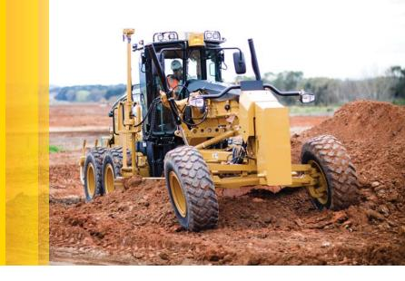
The Cat® 12M Motor Grader is designed to help you get more work done in less time with a 4.2 m (14 ft) moldboard. Unprecedented operator comfort and ease of service help to maximize your return on investment.
